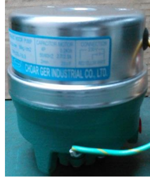
Hydraulic Motor 230V, 50Hz/2.7A, 60Hz/2.3A
