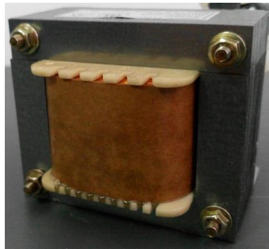
Linear Transformer 117V, 50/60Hz, 60W
